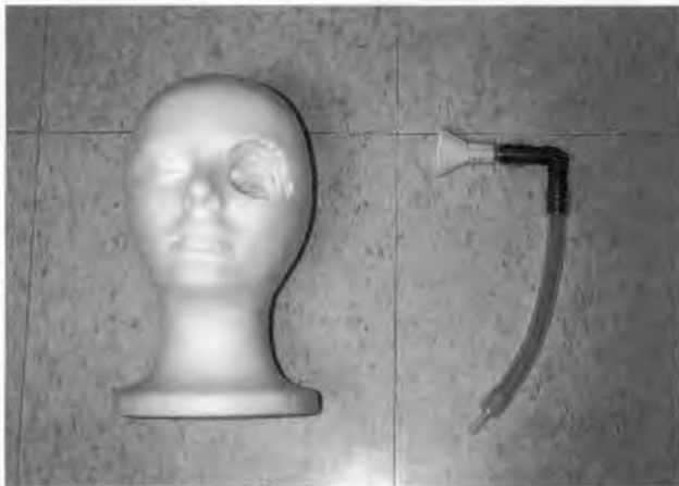
Figure 1. Modified Styrofoam head and vacuum tubing components of the device.
